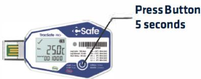
*If logger starts normally, green LED light will blink once every 10 seconds; If alarm is triggered, green LED light will STOP and red LED light will blink once every 10 seconds.*
